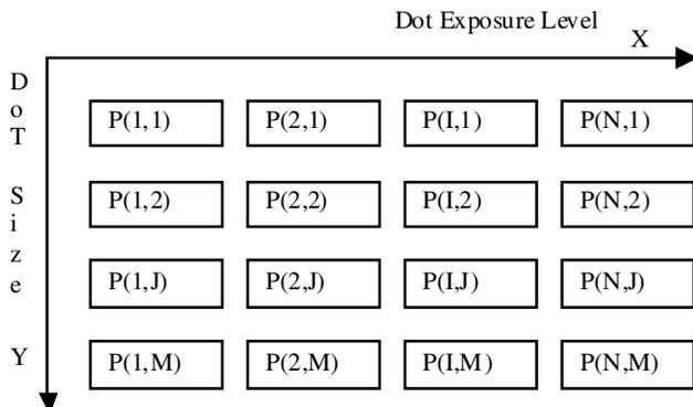
Figure 1. Illustration of Dot formation Chart. Each patch  $P(I,J)$  represents a dot formation at specific dot size and dot exposure.
