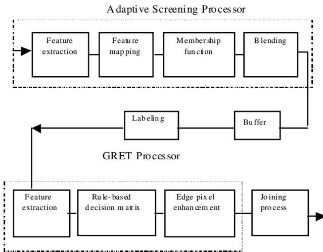
Figure 2. Functional diagram of the BEST algorithm.
