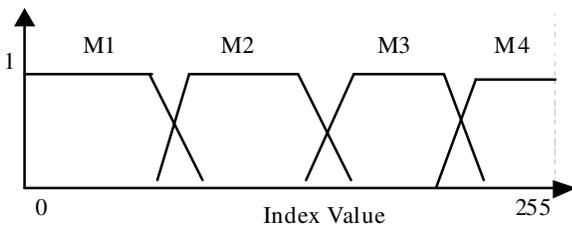
Figure 3. Illustration of typical membership functions of different dot types.
