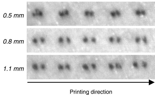
Figure 6. Dot shape in dependence of head-paper distance at constant speed (1.5 m/s)
