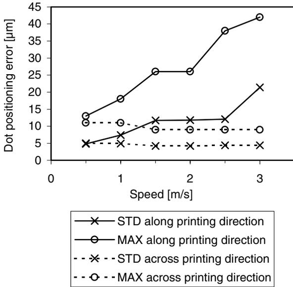
Figure 1. Dot positioning accuracy along printing direction for different speeds (STD: Standard deviation, MAX: Maximum deviation)
