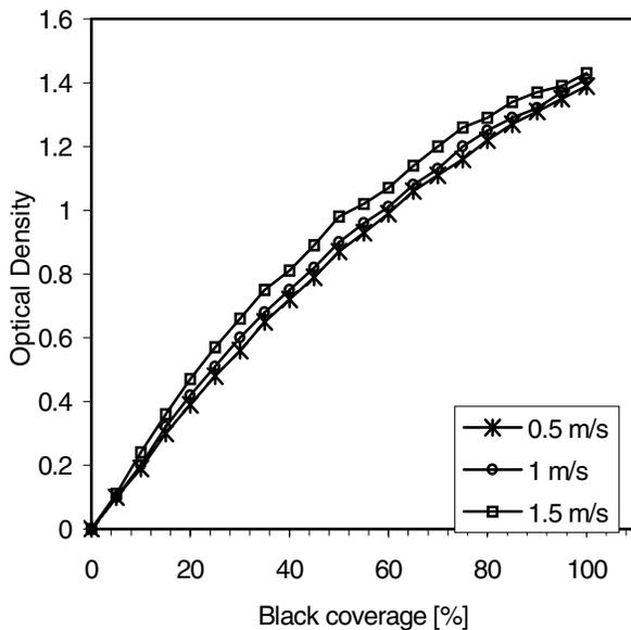
Figure 5. Optical density in dependence of speed and coverage
