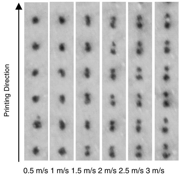
Figure 4. Dot shape in dependence of scanning speed
