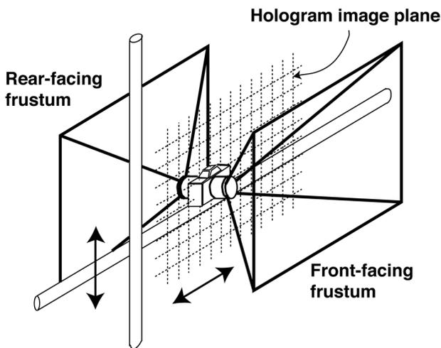
Figure 1. Hologram-centric double-frustum camera
