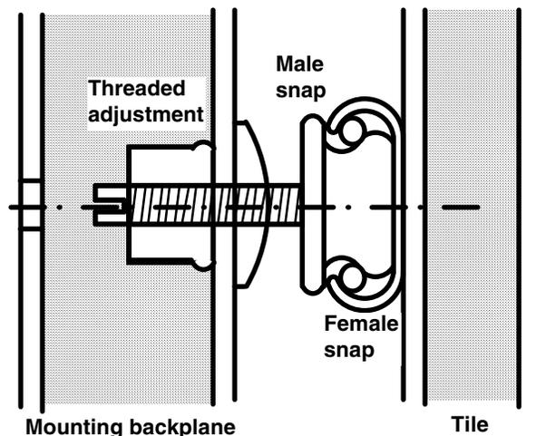
Figure 7. Adjustable tile mounting point.
