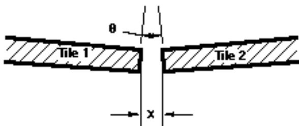
Figure 6. Tile-to-tile abutment and angular relationship.
