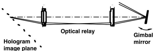
Figure 4. Reference beam-steering configuration.
