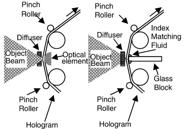
Figure 3. Reflection type head Figure 4. Edge-lit type head
