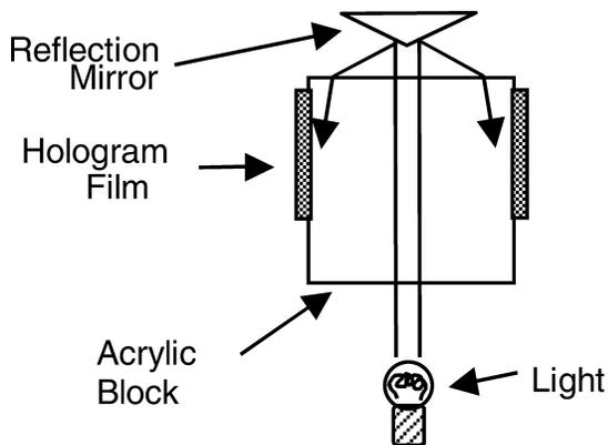
Figure 8. Cross section of a cylindrical edge-lit hologram viewer
