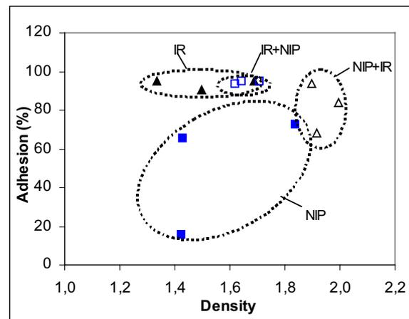
Figure 3. Example of fusing experiments with different combinations of nip and IR fusing.
