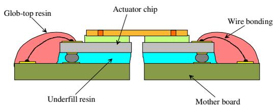
Figure 5. Wire bonding solution (CEA/LETI - 2)
