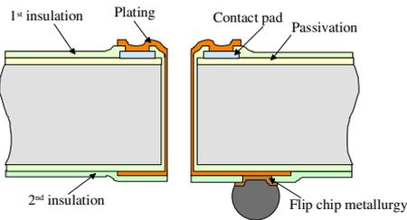
Figure 4. Feedthroughs solution (CEA/LETI - 1)
