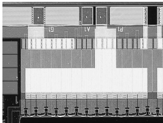
Figure 2. Printhead chip: view of a nozzle row
