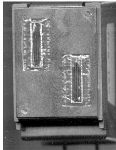
Figure 8. HSTACK printhead after stress test
