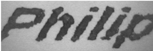
When the firing voltage decreased to reduce drop volume and improve dry time, incomplete fill was observed.
