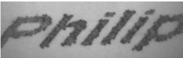
In the previous image the ink dries slowly and spreading and ink density variability are evident. By changing ink formulation, print quality improved as shown in the following, however drop volume and drying time were still excessive.
