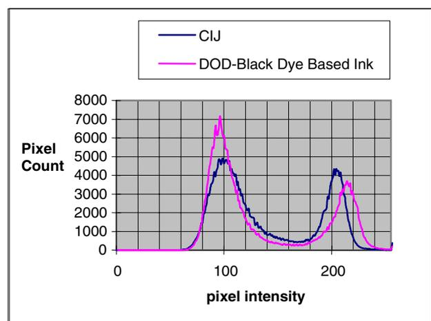
Figure 1. Contrast for CIJ and DOD1 prints on clay coated label at 50 fpm.
