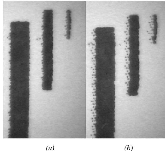
Figure 2. Print quality deterioration due to satellites. (a) 50 fpm, (b) 100 fpm.
