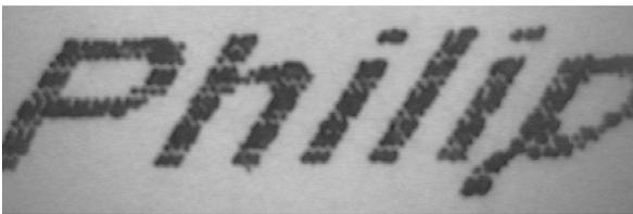
The best print with improved dry time was achieved by firing at the low voltage on a preheated substrate.
