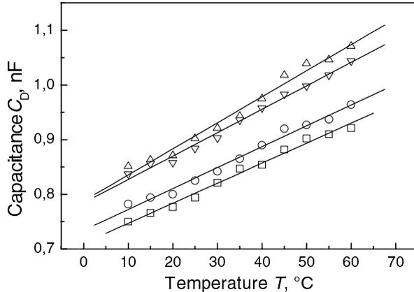
Figure 3. Electrical capacity of individual dummy walls versus temperature.
