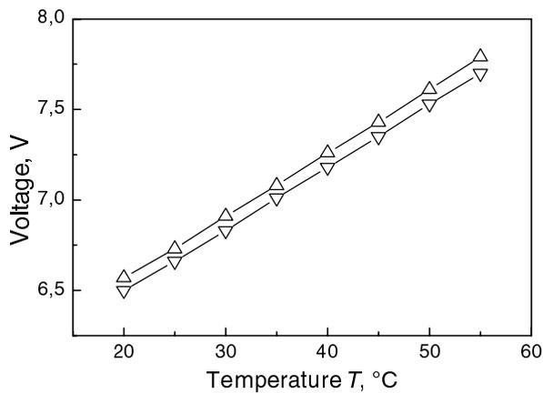
Figure 5. Typical calibration curves of dummy wall thermometers.
