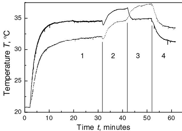
Figure 8. Temperatures at both ends of the actuator for different print pattern.
