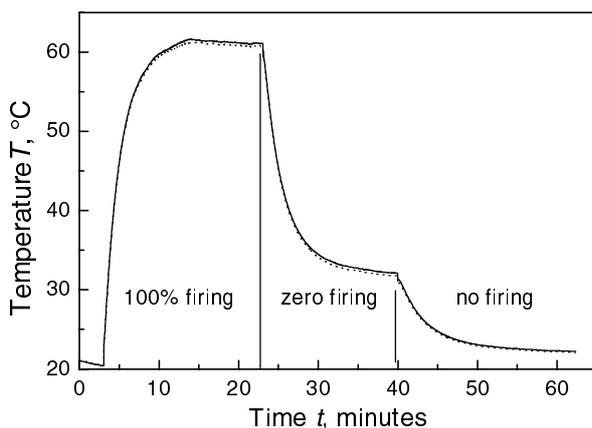
Figure 6. Temperatures at both ends of the actuator when printing without ink.
