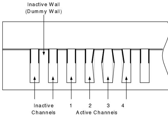
Figure 2. Actuator cross section and 'dummy wall'.
