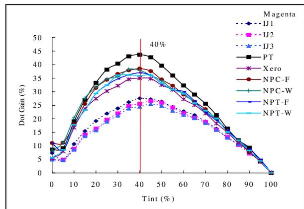
*Figure 1. Dot gain versus tint value of all paper samples with magenta ink*
