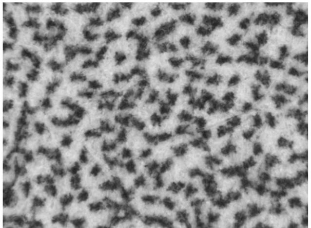
Figure 2b. High magnification image of the same halftone printed on a plain, uncoated substrate
