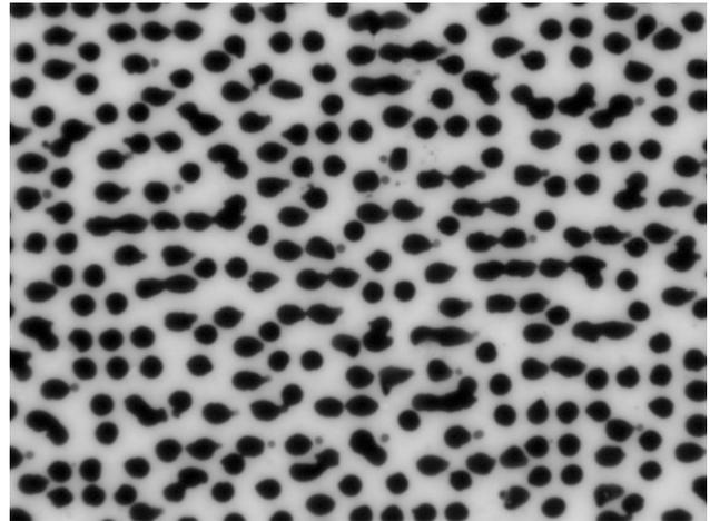
Figure 2a. High magnification image of a halftone printed on a glossy substrate
