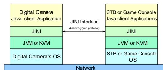
Figure 2. Communication with the JINI technology
