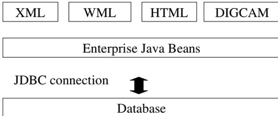
Figure 7. A typical Internet Imaging Server's Architecture
