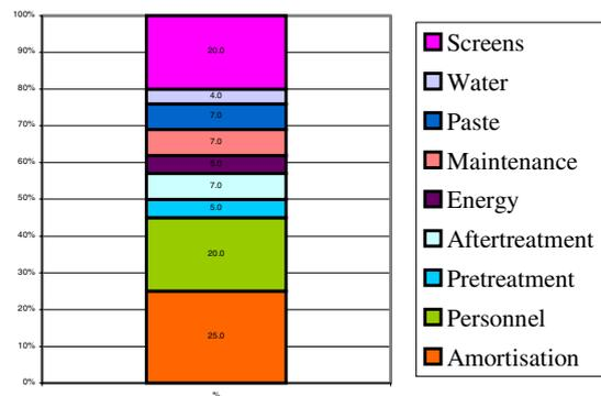
When comparing the cost between rotary screen printing and digital printing, for an average 10 colour print job and in function of the total printing length, following figures can be compared:
