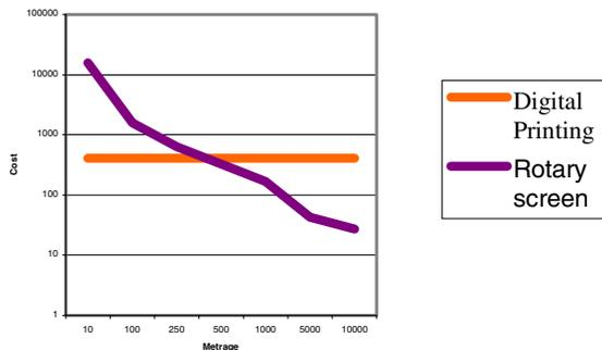
Here one can see that the breakpoint between rotary screen and digital printing lies around 400 meters. If the speed of the machines in digital printing increases faster than the price of the digital printing machines, then the amortisation and labour costs will become less important in relation to the other costs, which will very quickly push the break even point over 1000 meters.
