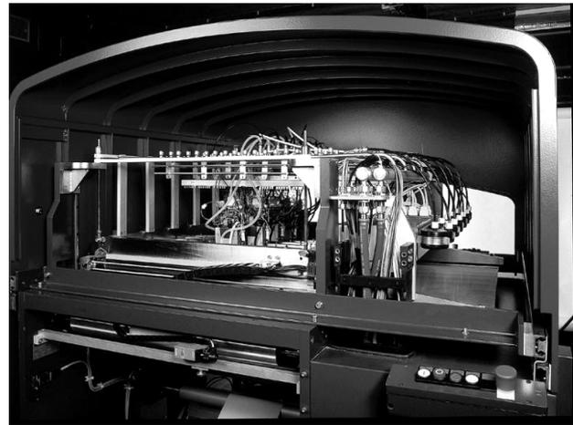
Barco has implemented a matrix of 9 cartridges to print the maximum print width of 63 cm. To obtain an invisible stitching the cartridges overlap. In real size the overlap is only some nozzles. Stitching is perfectly managed both in software and/or hardware.
