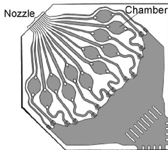
Figure 2. Conventional Piezo Head.
