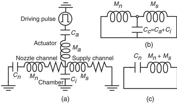
Figure 5. Equivalent model of the MLChip type MACH.
