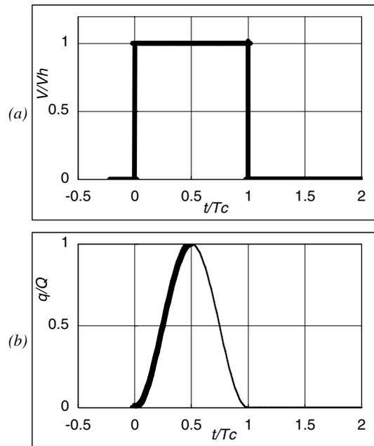
Figure 7. Push-Pull pulse (a) and response (b). Time in abscissa is normalized by  $T_c$ , and also voltage and flow quantity in ordinates are normalized by the pulse height and flow amplitude respectively.
