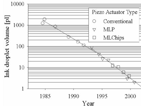
Figure 1. History of ink droplet volume of EPSON's piezo type printers.
