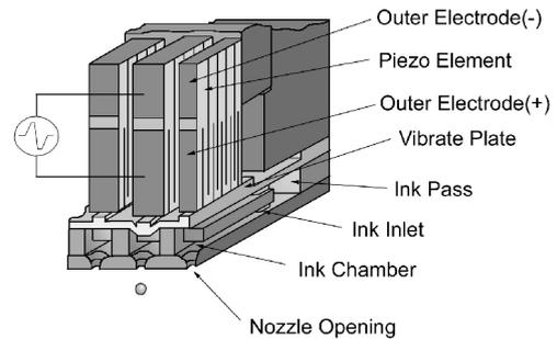
Figure 3. Structure of the MLP type MACH
