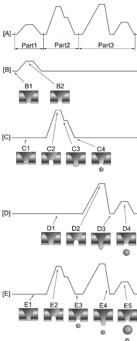
Figure 10. Driving waveform of MSDT
