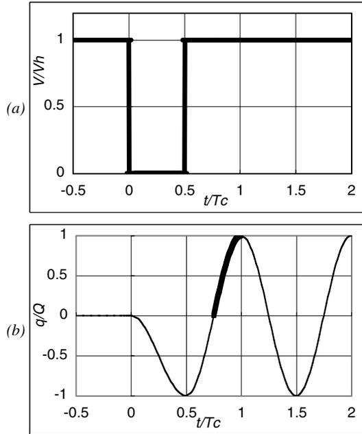
Figure 8. Pull-Push pulse (a) and response (b).
