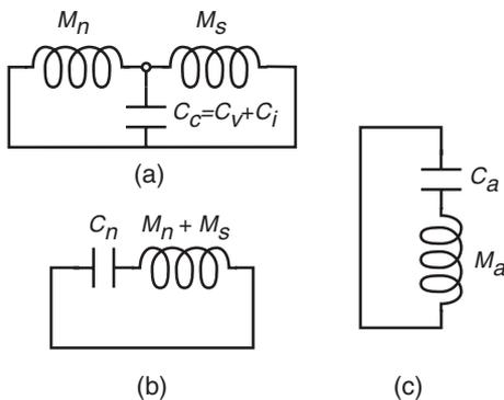
Figure 6. Equivalent model of the MLP type MACH.
