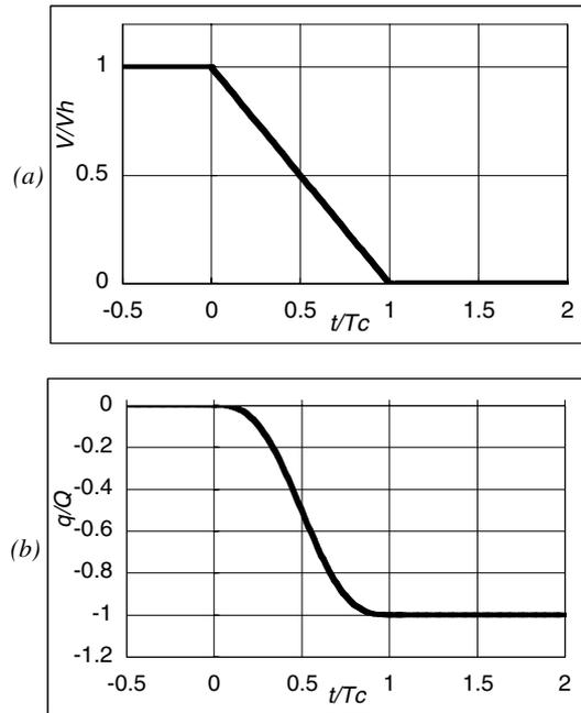
Figure 9. Ramp step input (a) and response (b).
