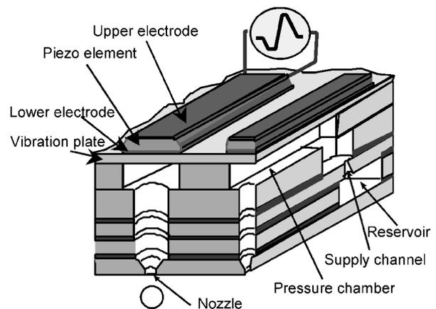
Figure 4. Structure of MLChips type MACH.
