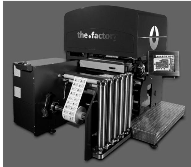
*the.factory industrial drop-on-demand inkjet press. Uses up to 6 UV-curing inks and has a maximum web speed of 21m/min.*
