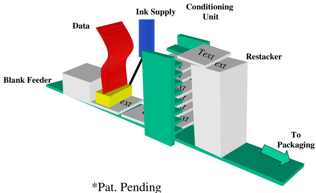
Figure 1. Schematic of the prototype printer for printing variable information on packages.
