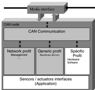
Figure 2. Network node architecture
