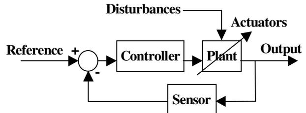
Figure 1. Basic control system block diagram
