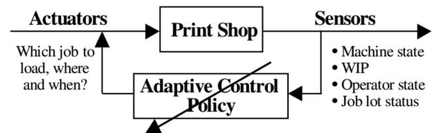
Figure 2. Schematic description of a feedback control structure applicable to print shop operations.
