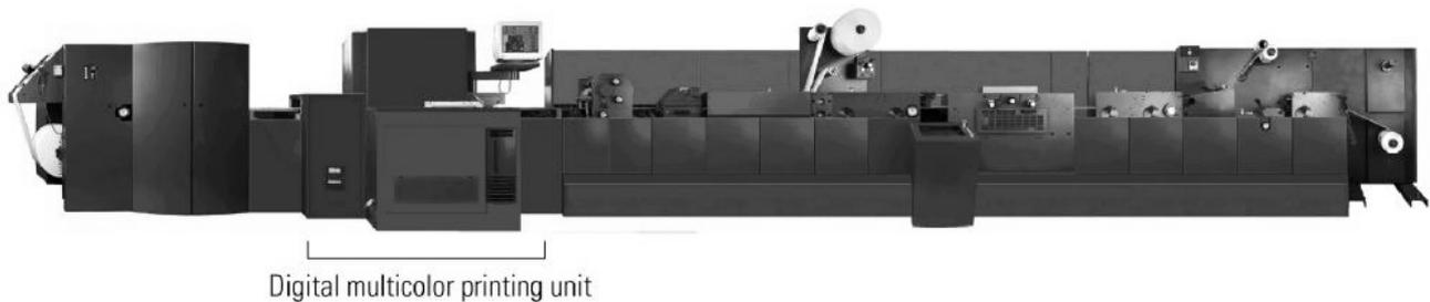
Figure 8. Digital label printing system with NIP-multicolor printing system (electrophotography with liquid toner; Omnius, Indigo), flexographic printing, and finishing equipment for coating, laminating, and die-cutting (DO 330, Gallus/Indigo)
