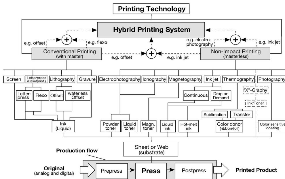
Figure 1. Combination of various printing technologies to set up hybrid printing systems.<sup>1</sup>
