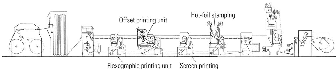
Figure 3. Hybrid printing system for label printing combining flexography, offset and screen, as well as letterpress for hot-foil stamping/embossing (CombiPrint, Goebel/Drent)<sup>1</sup>
