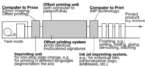
Figure 9. System study: components of a digital hybrid printing system for web-fed printing for the production of segmented, personalized/individualized print media.<sup>1</sup>
