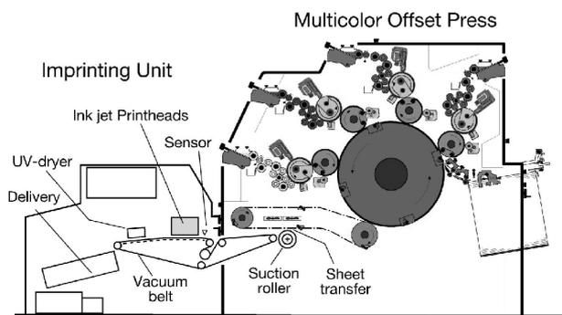
Figure 5. Digital hybrid printing system using the combination of offset and ink jet technology (Heidelberg)
