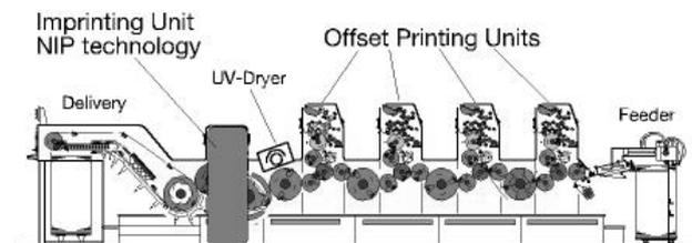
Figure 7. Hybrid printing system combining offset printing for multicolor printing with NIP-technology for the imprinting unit to produce partly variable contents from sheet to sheet (Heidelberg)
