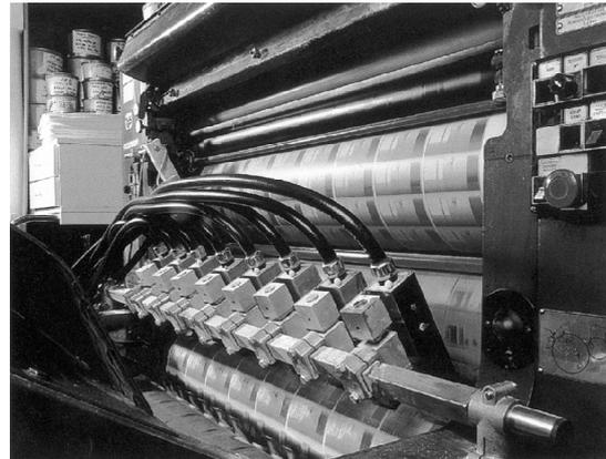
Figure 6. Hybrid printing system: Multicolor offset printing press with ink jet imprinting system for numbering, personalization, addressing and segmentation of the job (Domino/Heidelberg)
