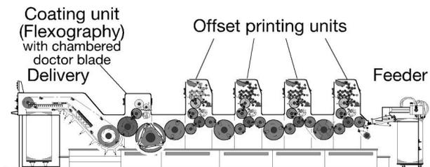
Figure 2. Multicolor sheet-fed offset press with coating unit as a hybrid printing system combining offset and flexographic printing
