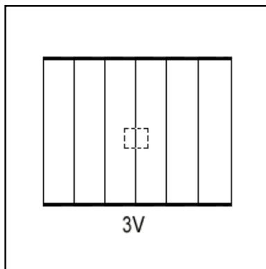
Figure 5: Modified test target with FOV rectangle superimposed
