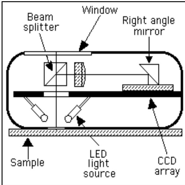
Figure 1: Measurement head assembly schematic
