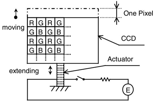
Figure 2 One-dot-movement mechanism.
