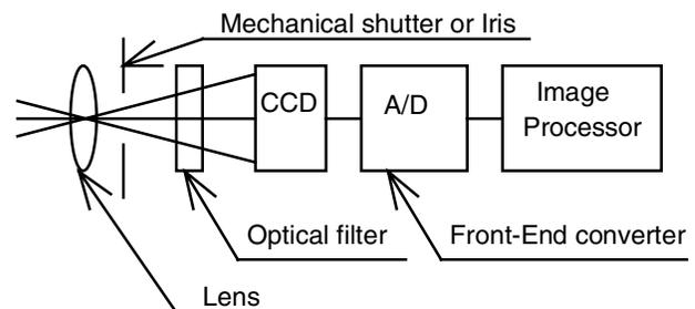
Figure 1 Digital camera's configuration.
