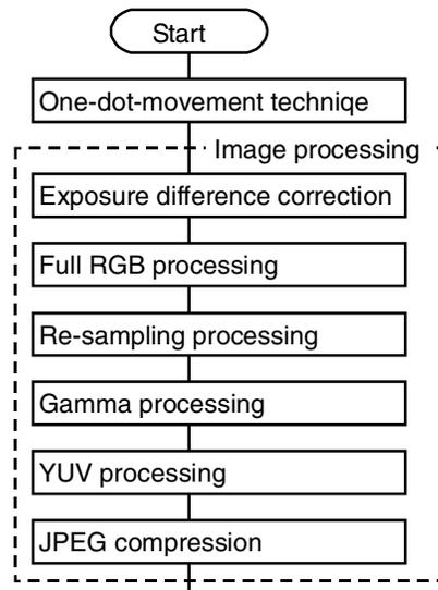
Figure 4 Flow chart of image processing.
