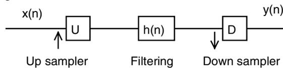
Figure6 Block diagram of re-sampling.
