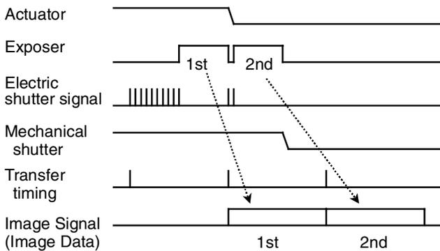
Figure 3 Timing chart of using full frame CCD.
