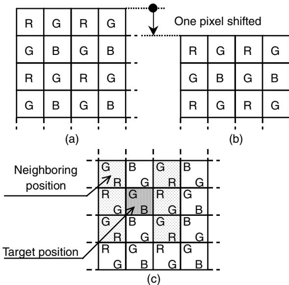
Figure 5 Color image of Full RGB processing: (a) 1st image, (b) 2nd image, and (c) 1st and 2nd Image.
