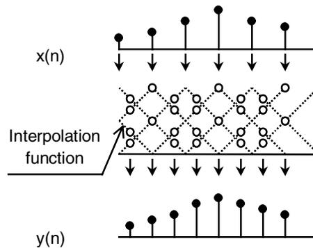
Figure 7 Re-sampling by using the interpolation function.
