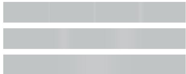
*Figure 2 - 3 uniform patches with equal amplitude streaks of different widths. First row has a 0.5 mm, 1 mm, and 2 mm wide streak. Middle patch has a 5 mm and 10 mm wide streak. Bottom patch has a 20 mm wide streak.*
