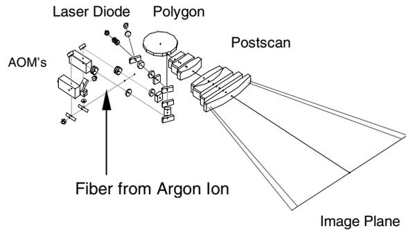
Figure 1. Laser Recorder Unit of Agfa Digital Minilab
