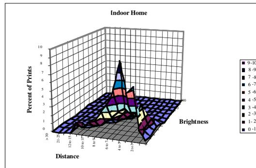
Figure 3. Photographic utilization space for a 35 mm single lens reflex camera under indoor illumination conditions.
