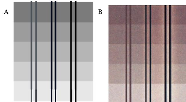
Figure 1. Example of test elements used for HDST evaluation. (A) Digital original; (B) Scan of print sample. The HDST defect is most clearly seen as the light halo surrounding the right most line-pair in (B).
