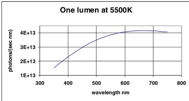
Figure 6. Photons/sec-nm at 1 lumen
