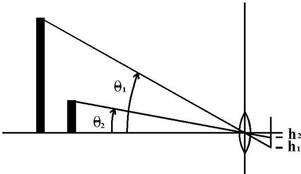
Figure 1. Unit angular magnification
