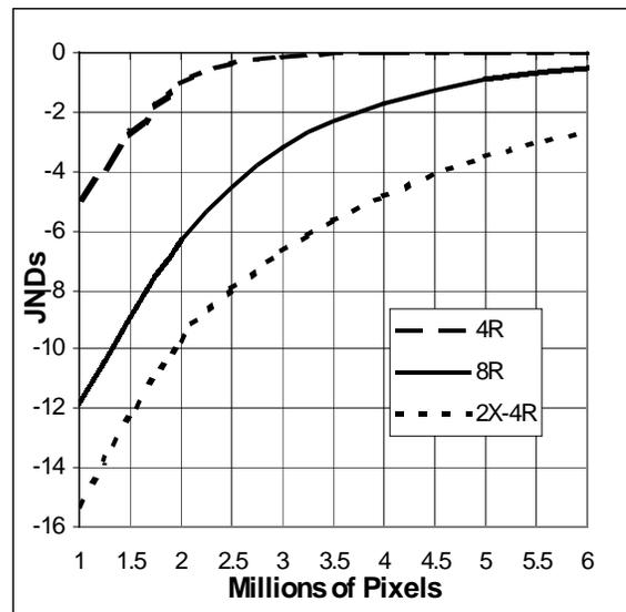
Figure 5: Determination of digital still camera pixel number requirements for various print sizes
