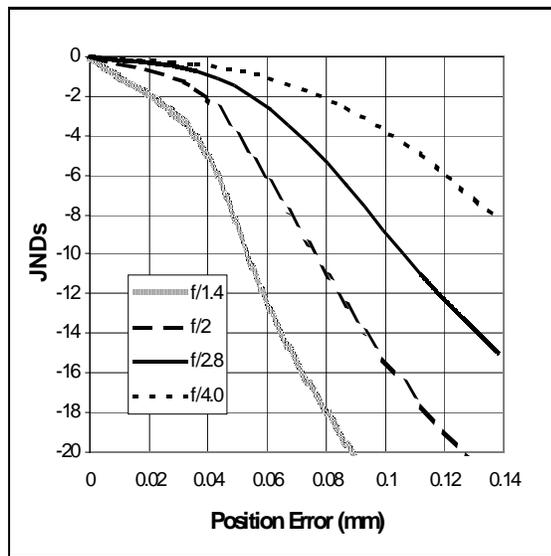
Figure 6: Determination of digital still camera optical positioning tolerances
