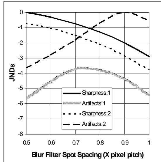
Figure 7: Selection of blur filter spot separation
