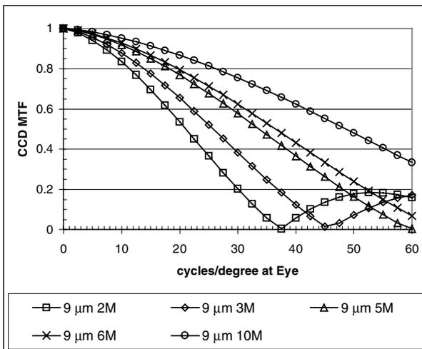
Figure 2. CCD aperture MTF scaled for viewing
