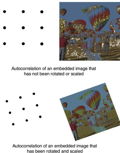
Figure 6. The concept of autocorrelating an embedded image to derive scale and rotation parameters
