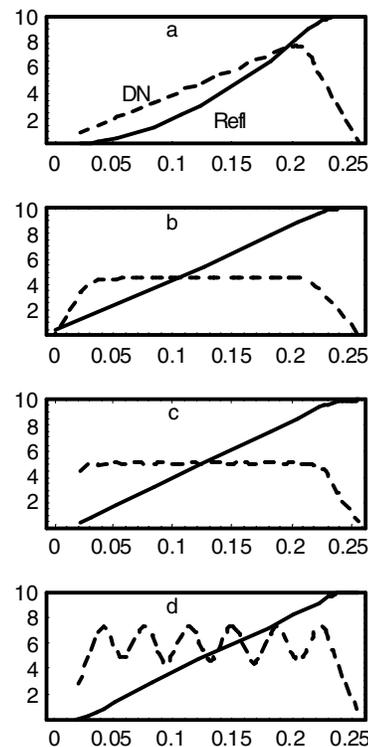
Figure 2. Reflectance (solid) and noise (dashed) characteristics corresponding to DQE characteristics of figure 1.
