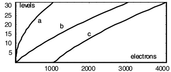
Figure 4. Sampling function, electrons to digits. a)  $2\sigma$  criterion, photons alone, b) overall  $2\sigma$  criterion applied, including spurious noise, c) sampling offset according to spurious noise.
