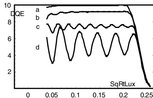
Figure 1. DQE-exposure characteristics for four digitization schemes. a) every electron, b)  $1\sigma$ ; c)  $2\sigma$ ; d)  $3\sigma$ -criterion.
