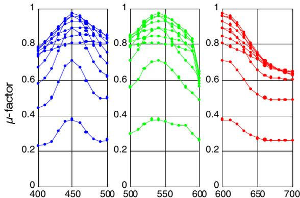
Figure 6.  $\mu$ -factor of a set of ss: one ss changes peak  $\lambda_0$ , the other two ss fix peak  $\lambda_0$ , that is, change one of (450nm, 540nm, 600nm) by 10nm and vary width from 10nm to 100nm by 10nm
