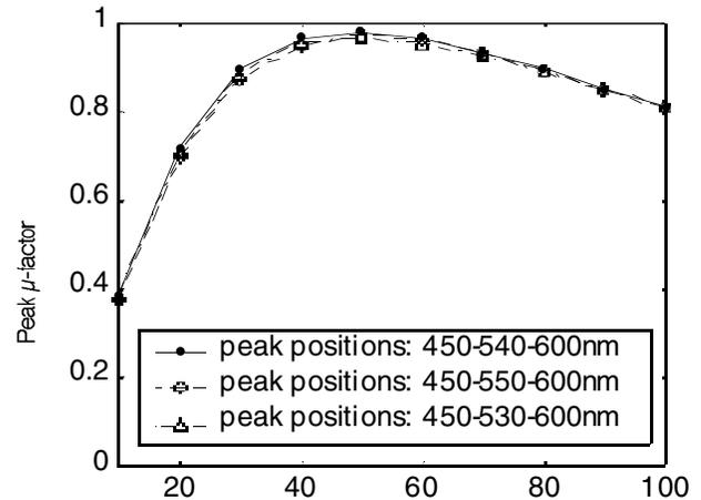
Figure 5. Effect of width of  $SS$  on peak  $\mu$ -factor Optimal width is about  $w=45\sim 55nm$
