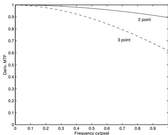
Figure 4. MTF caused by computation the edge gradient by a finite difference. The 3-point difference  $[-0.5 \ 0 \ 0.5]$  is used in the ISO procedure.
