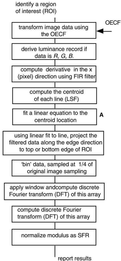
Figure 2. Description of the ISO 12233 spatial frequency response evaluation method. The edge is assumed to be oriented in a near-vertical direction.
