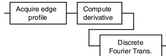
Figure 1. Edge-gradient analysis steps
