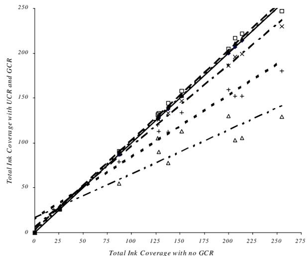
Figure 2: Effect of GCR on Total Ink Coverage for Average Key Image
