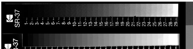
Picture 2. Halftone Rendered Test Target
