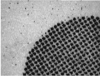
*Picture 5. Magnified Traditional Screened Output*
