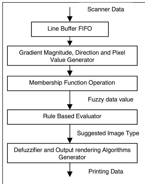
Figure 1. Block Diagram of Rule-based Segmentation Algorithm
