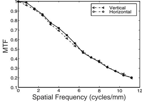
Figure 7. MTF from step images printed on glossy coated paper in vertical and horizontal printing direction.
