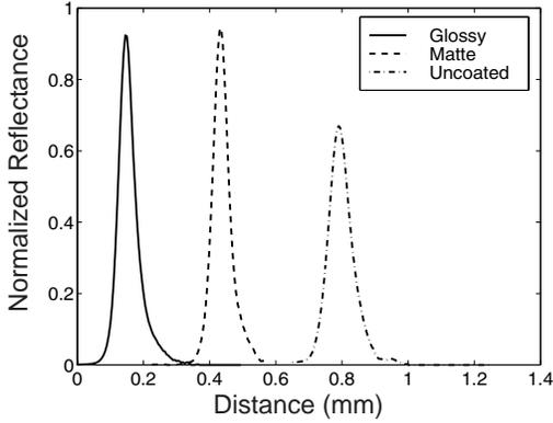
Figure 4. Line spread function from step images printed on glossy coated paper.
