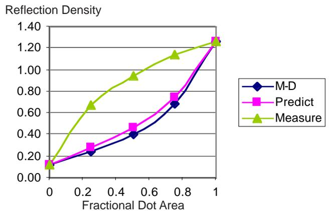
Figure 13. Reflection density of line screen 180 lpi printed on uncoated paper.
