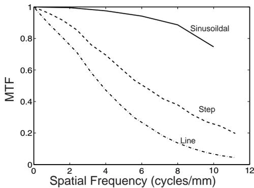
Figure 5. MTF from sinusoidal, one-pixel line and step image printed on glossy coated paper.
