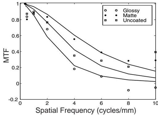
Figure 8. MTFs from contact sinusoidal pattern film on glossy, matte and uncoated paper. The solid lines are MTFs calculated by the model with  $d$  values 0.052, 0.025 and 0.035 respectively.
