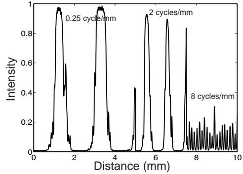
Figure 2. Intensity trace from sinusoidal image at spatial frequency 0.50, 2, and 8 cycles/mm printed on glossy coated paper.
