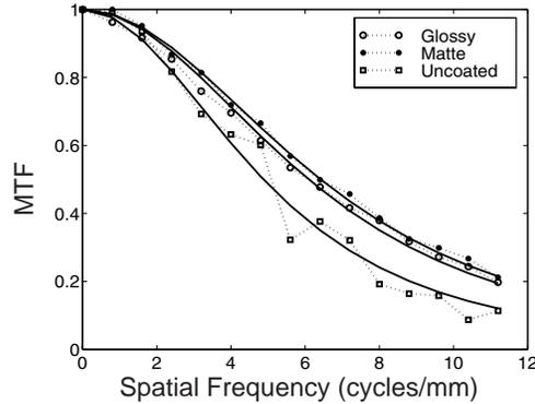
Figure 6. MTF from step images printed on glossy coated, matte-coated and uncoated paper. The solid lines are MTFs calculated from model in Eq. (9) with  $d=0.020, 0.19$  and  $d=0.025$  for glossy, matte and uncoated paper respectively.
