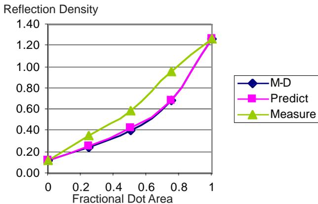
Figure 11. Reflection density of line screen 45 lpi printed on uncoated paper.
