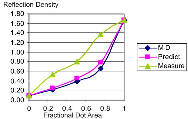
Figure 12. Reflection density of line screen 180 lpi printed on matte-coated paper.
