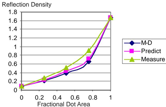
Figure 10. Reflection density of line screen 45 lpi printed on matte-coated paper.
