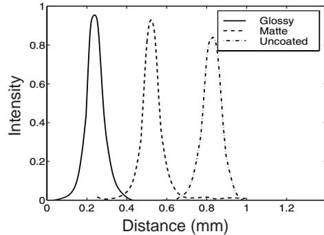
Figure 3. Line spread function from one-pixel line images printed on glossy coated paper.
