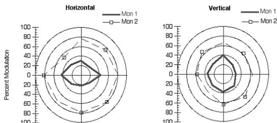
Figure 3. Comparison of horizontal and vertical modulation values as a function of screen position.
