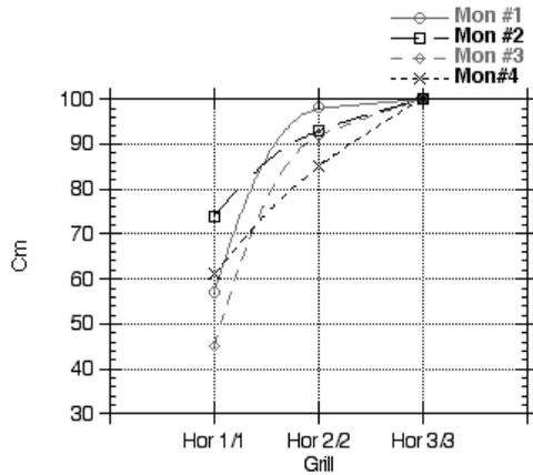
Figure 2. Effect of grill size on horizontal  $C_m$
