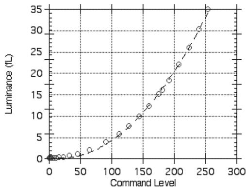
Figure 1. Typical command level/luminance function
