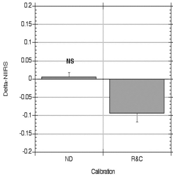
Figure 8. Delta-NIIRS ratings for NEMA/DICOM and Rogers and Carel calibrations relative to IDEX calibration.
