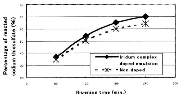
Fig.1 Effect of iridium complex doping on reactivity of sodium thiosulfate sensitizer during chemical ripening
