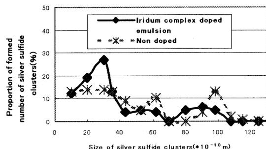
Fig.2 Effect of iridium complex doping on size distribution of silver sulfide clusters after chemical sensitization by sodium thiosulfate
