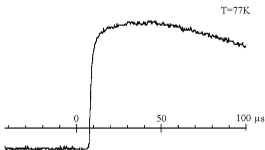
Figure 5. Time dependence of the microwave absorption signal at 77K for the sample as in Fig. 3, lower trace
