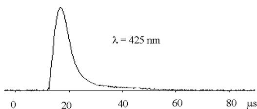
Figure 2. Time response of the flash used for photo excitation
