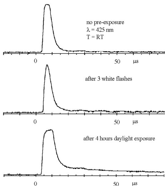
Figure 3. Time dependence of absorption signal after different exposures of the film
