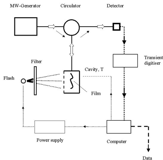
Figure 1. Schematic diagram of the apparatus for microwave detected PICTS
