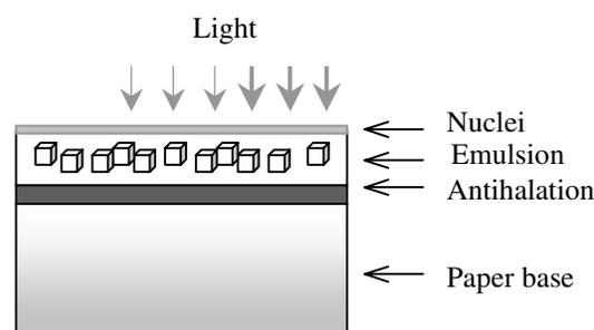
Fig. 1 Cross section of CTP printing plate
