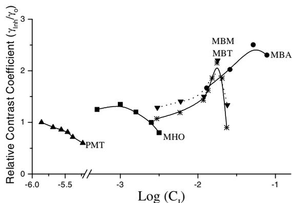
Fig. 4 Effects of inhibitors at different concentrations on relative contrast coefficients
