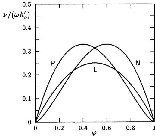
Figure 7: The shift of the Maximum Yule-Nielsen Effect: For linescreens (L) a centered curve with a apex of 0,5 is calculated, for negative (N) and positive (P) cylindric dots with shifting apex's.
