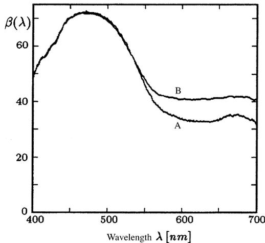
Figure 4. Spectral Deviations by the Yule-Nielsen Effect: The measured spectrum A is different to the predicted spectrum B which is calculated as the sum of the plain paper spectrum and the solid tint spectrum without correction for the Yule-Nielsen effect (Cyan raster with  $\varphi = 0,53$ ).
