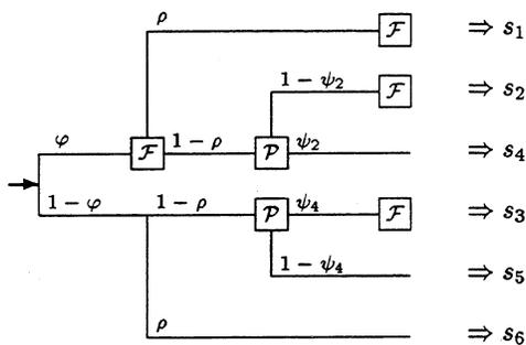
Figure 2. Structure of the Light Paths: There are six fundamentally different pathes, each with its own shares  $\varphi, \psi, \rho$ .
