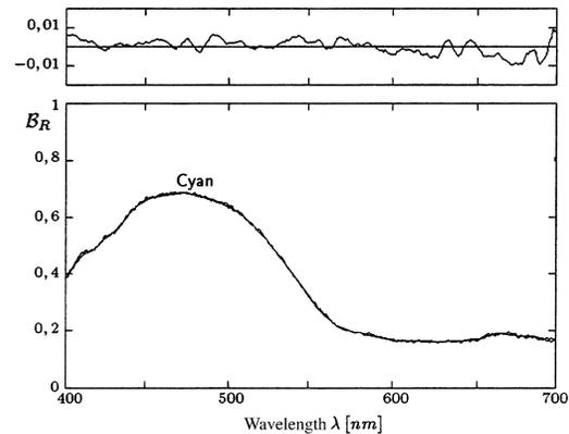
Figure 6: Measured and Calculated Spectrum: The two spectra in the bottom plot overlay each other as near equivalents. In the upper plot the difference between the measured and calculated curve is shown on an enlarged scale.
