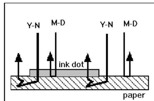
Figure 1. Light Pathes in a Screened Image: (M-D) signifies the light pathes assumed by Murray-Davies, while (Y-N) shows the horizontal light scattering in the paper discovered by Yule-Nielsen.
