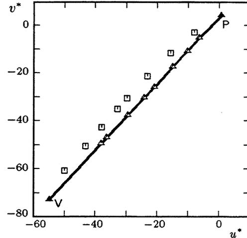
Figure 5. Plot of the color coordinates for different geometrical area coverages in the  $L^*u^*v^*$  color space. The direct line between plain paper (P) and the solid tint (V) is the uncorrected prediction, the measured curve shows the influence of the Yule-Nielsen effect.
