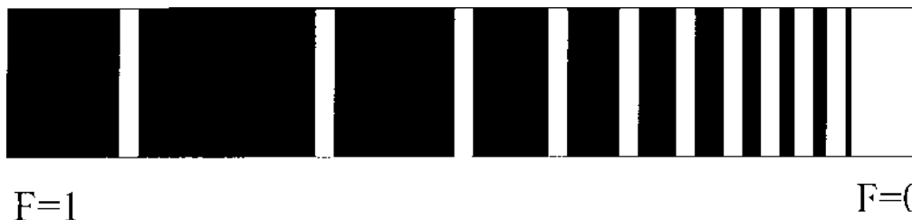
Figure 13. Illustration of a halftone line pattern that is FM in terms of the spaces between the lines, but AM with respect to the lines.
