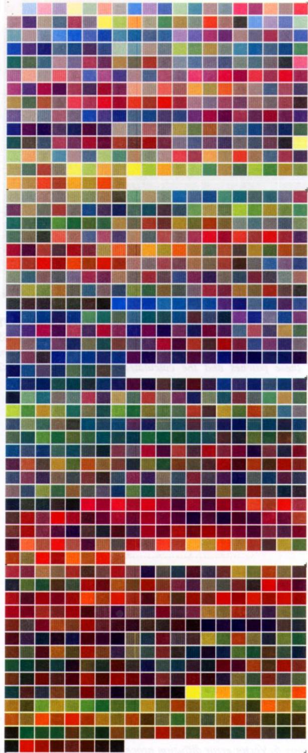
Figure 4. One thousand and seventy-two  $2 \times 2$  patches printed by a Xerox 5790 color laser printer in  $400 \times 400$  DPI mode. A CIE XYZ look-up table is generated from color measuring and used for the algorithm-independent color calibration.
