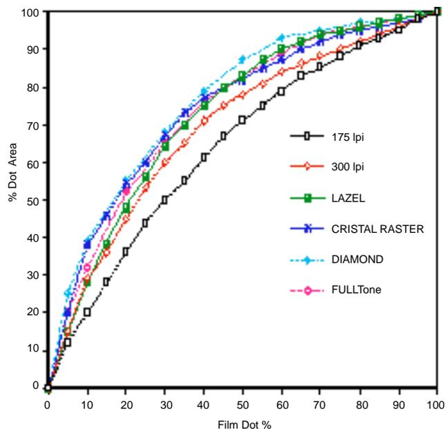
Figure 2. % Dot Area Curves for Commercial Stochastic Screen Algorithms
