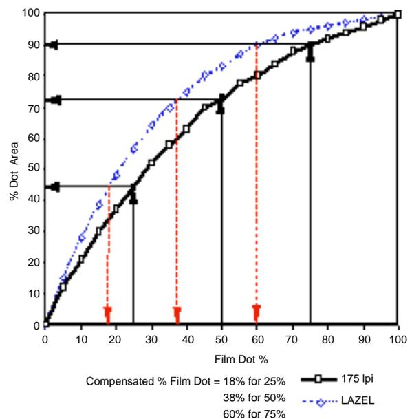
Figure 3. Dot Gain Compensation for Stochastic Screening
