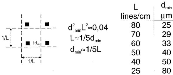
Figure 2. With a various screen rulings the approximately 4% highlight dot is used which expresses the empirical alternative in providing two dissimilar and conflicting properties of a halftone image
