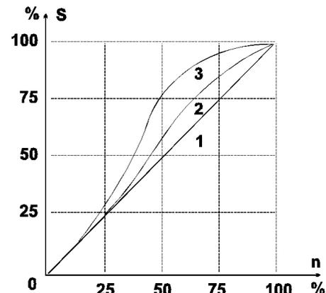
Figure 5. Coverage "S" nonlinear relates to the number "n" of randomly located microdots due to the additional inked areas formation when adjacent microdots contact each other: 1 at idealistic (bit-map) presentation; 2,3 at low and high recording resolution.
