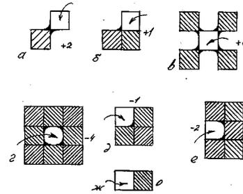
Figure 4. Dot gain value depends on printed area geometry as producing from +8 to -4 extra inked areas with a single microdot (not hatched) addition.
