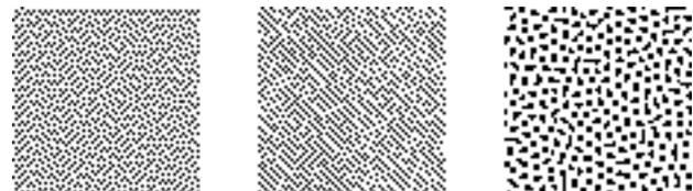
Figure 4. Three different halftones representing the very same gray level. The amounts of micro dots are the same but due to different structure properties, their appearances are totally different.
