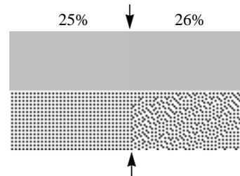
Figure 3. An enlargement of an undesired structural change in the halftone. The border between the two gray levels in the original is hardly noticeable but has been emphasized in the reproduction.
