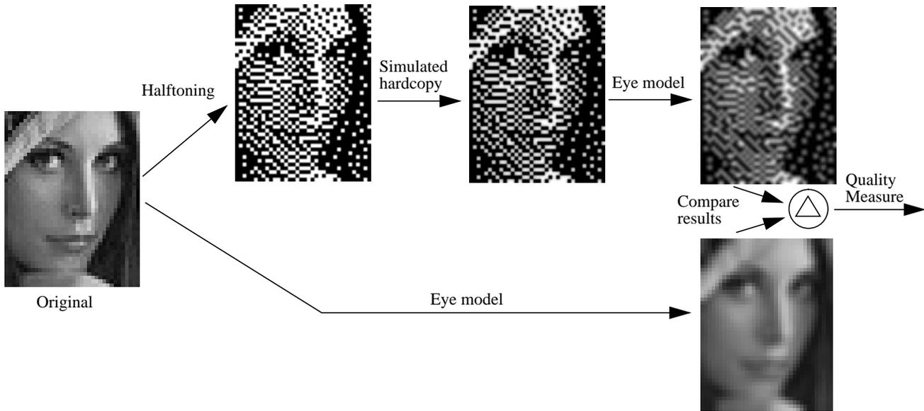
Figure 2. The principle of the model. The original is halftoned and the mechanical and optical effects when printed is added. The eye model is applied both on the original and the 'printed' image. The two results are to be evaluated by the quality measures.
