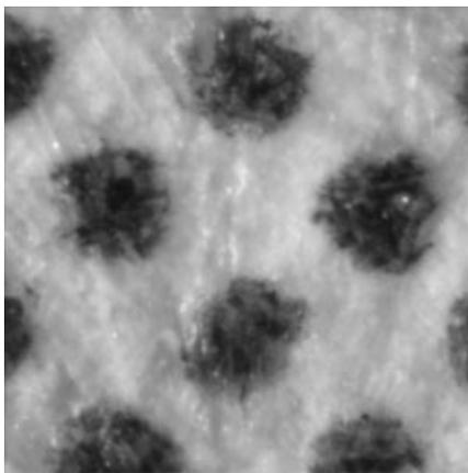
Figure 1. A microscope image of halftone dots printed on paper. The dots have rugged edges and have been spread outside their intended borders
