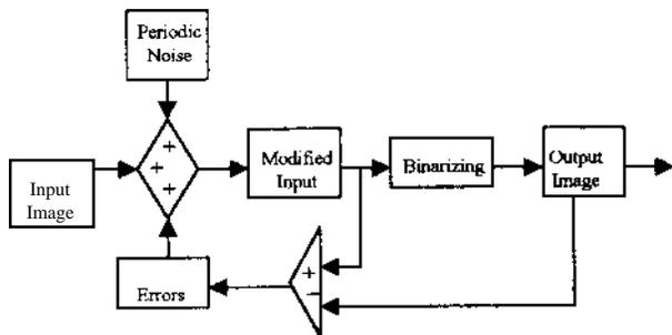
Figure 3. Graphical representation of proposed algorithm
