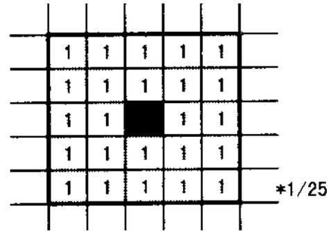
Figure 4. The averaging filter to decide the amplitude of the periodic noise
