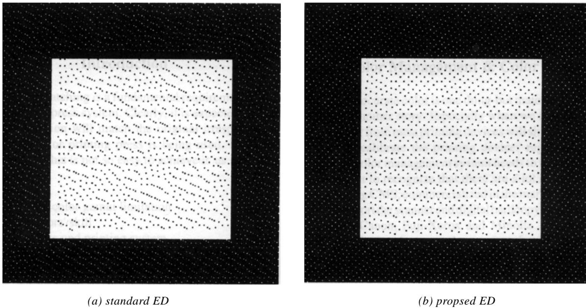
Figure 7. Binary images applied to a set of patches with gray levels "247" in highlight and "15" in shadow.
