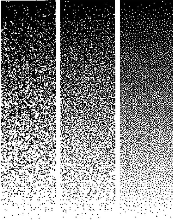
Figure 2. Halftone patterns generated by three  $64 \times 64$  stochastic halftone screens, respectively. a) The left column, by the initial screen of an optimization. b) The middle one, by a screen saved after 5,000 swaps. c) The right one, by a screen optimized in ten minutes with 1,000,000 swaps.
