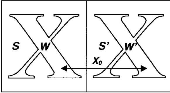
Figure 4. Configuration of a watermark halftone screen. The two watermark regions,  $W$  and  $W'$ , are identical in shape and separated by a distance  $X_0$  equal to a half of the screen width.
