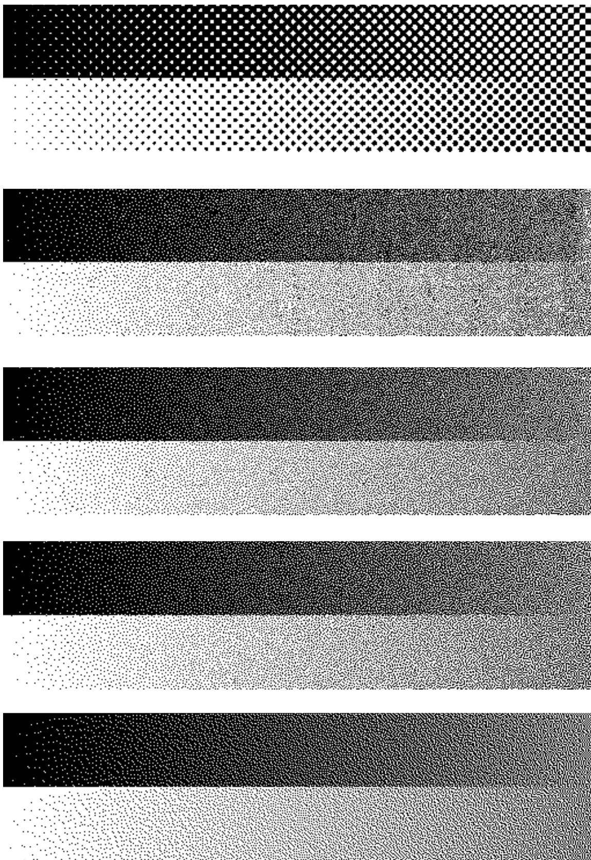
Figure 1. The original image is a 256-step gray-level wedge where every tint is 4 pixels wide. The wedge has been halftoning using: a) Conventional clustered dot halftoning, b) Optimized maps without correlation, c) Interpolation between optimized maps (Method 2, described in text) d) Optimized and correlated maps (Method 2, described in text) e) A commercial available Error Diffusion method.<sup>6</sup>
